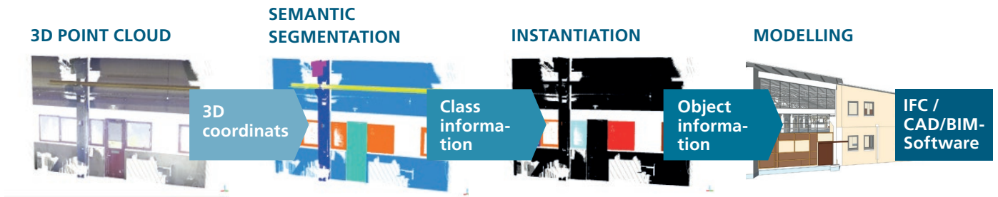
From point cloud to 3D model: In an automated process, point clouds are converted to semantically enriched models.
